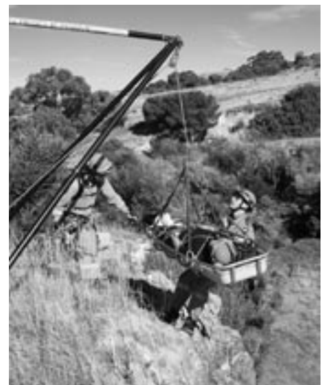
Stretcher rescue with injured person being hauled up a cliff using the Larkin Rescue Frame with the lift/lower systems to effect a safe rescue.
